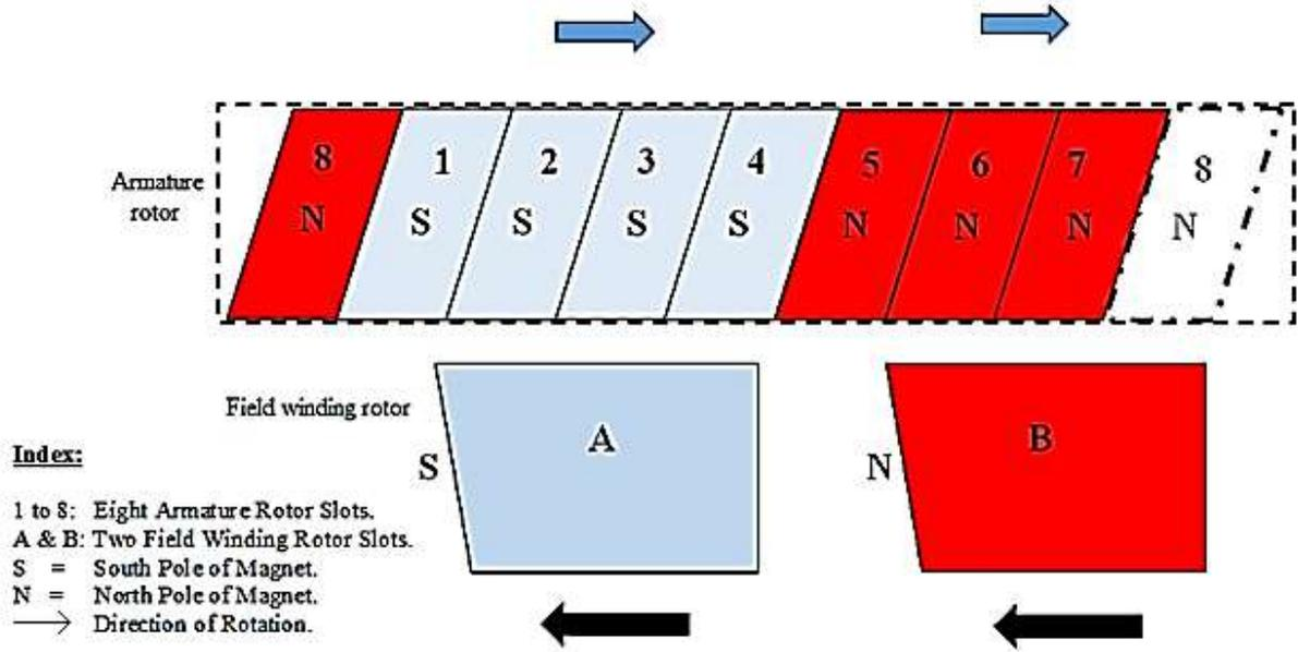
Figure A1. Armature and field winding rotors
