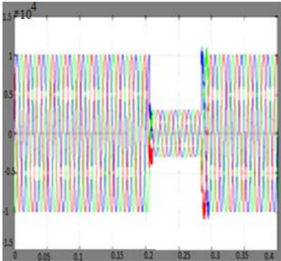
Figure 7. Source voltage under fault causing voltage sag
