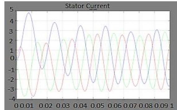
Figure 9. Stator current wave form
