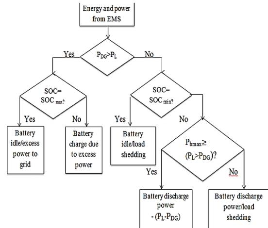
Figure 2. Battery operation in islanded mode
