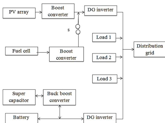
Figure 1. Block diagram of a micro grid
